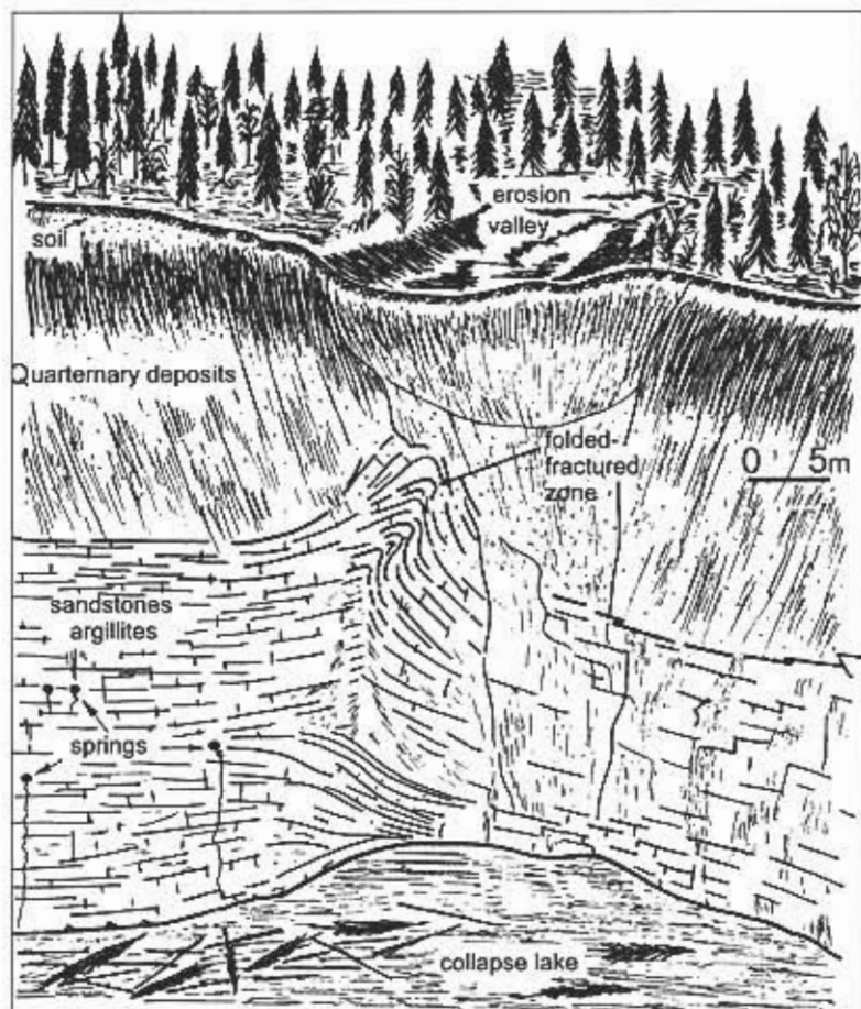
Fig.5 – Sketch of the northwestern side of the Berezniki Collapse (June, 1987). Arrows point to the fold deformation in the variegated complex
